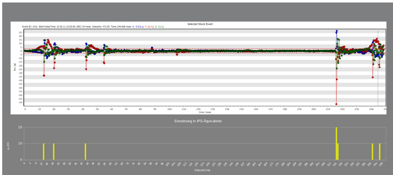
Fig. 3: 250 ms section of a measurement curve with resulting load in IPS
